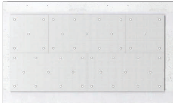
Figure 1.3. Board joints staggered
